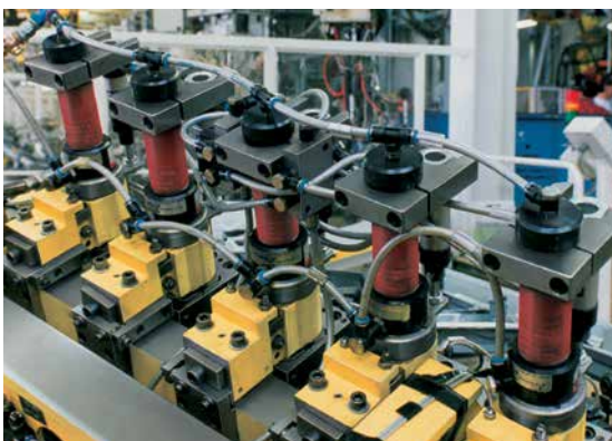
Stamping units placed in line
